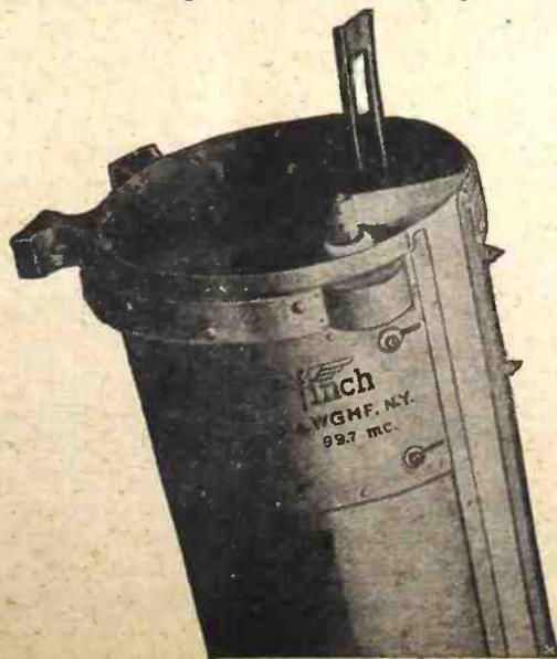
Close-up view of the new facsimile antenna.
